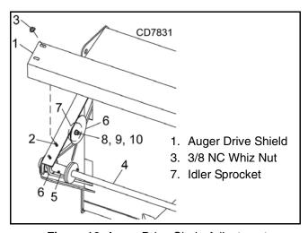
Figure 10. Auger Drive Chain Adjustment
